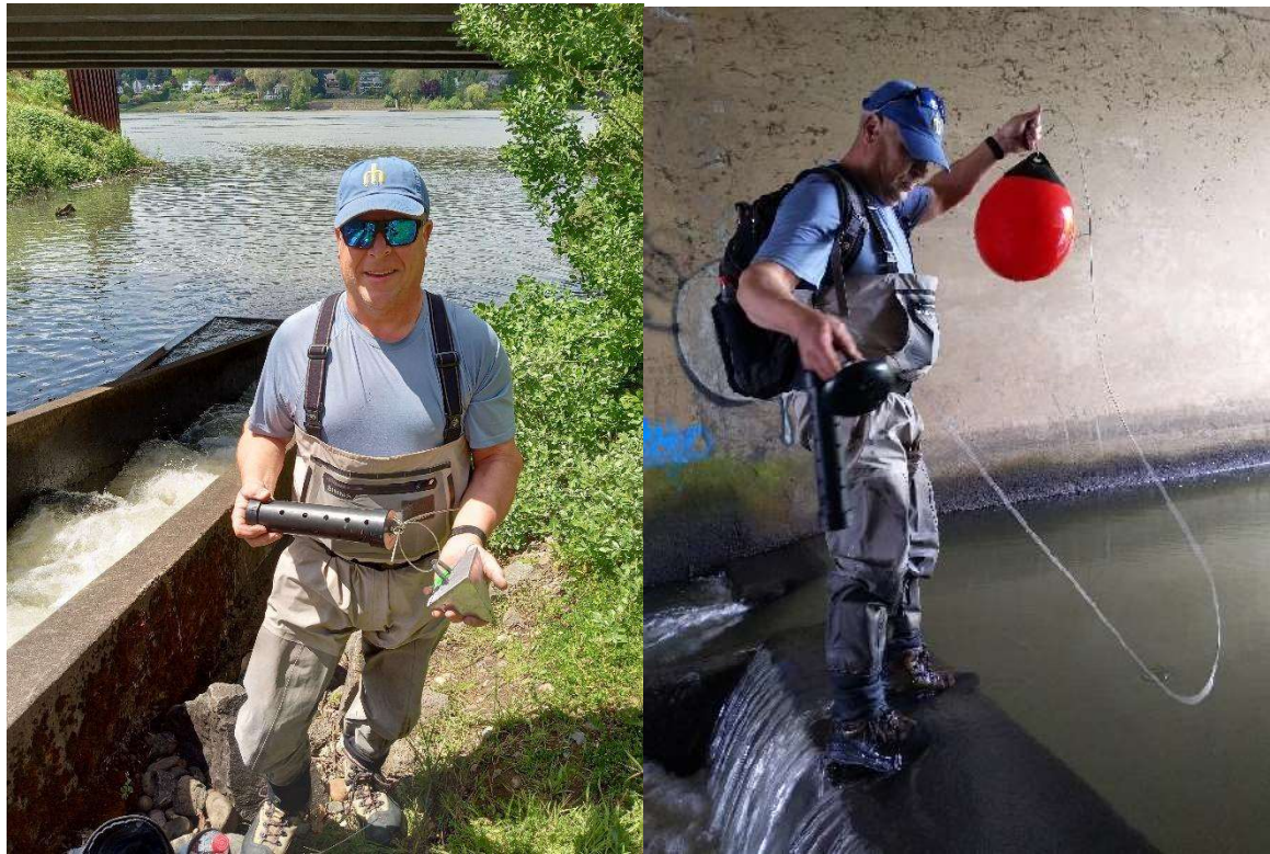
Figure 3 - Two different methods were used to install loggers at Kellogg Dam. In the fish ladder (left photo) the unit was submerged using a 10-pound weight. In the impoundment (right photo), the logger was attached to an anchor that was marked with a buoy.
